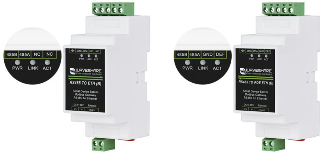
These two versions are the same in software functions, while RS485 TO POE ETH (B) is the hardware upgrade version, support PoE Ethernet port power supply, with power and signal isolation protection, which is safer for industrial applications.
