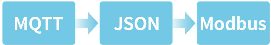
When used as MQTT gateway, the devices can upload serial data to MQTT server by MQTT protocol through transparent transmission, supported servers including Baidu Cloud MQTT, Alibaba Cloud MQTT, China Mobile OneNet, etc. The acquired Modbus RTU or non-standard serial data can be parsed into JSON format and packaged into MQTT data packet for uploading.
