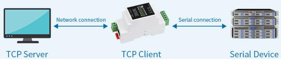
TCP Client will try establishing TCP connection with configured IP to achieve bi-directional transparent transfer between the server and serial device, and keeps retrying if failed
