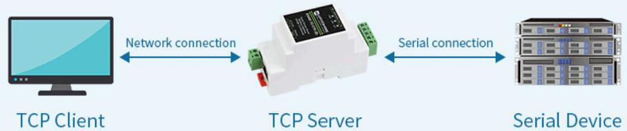
TCP Server will be listening configured ports and waiting for TCP Client connections, data from the serial device will be transferred via TCP Server to every connected clients
