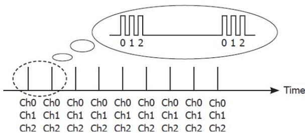
The I-8014W/I-8014CW module includes a 4 k sample onboard FIFO buffer for A/D conversion. The new FIFO technology uses a trigger interrupt signal, meaning that if the sampled count is higher than the pre-defined FIFO level, an interrupt signal will notify the host.
