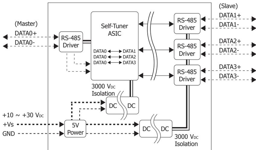
The following block diagram shows how I-7513 was designed as independent channel. Data coming from the master input will be transmitted to all four RS-485 slave channels. But data coming from the slave channels will be returned to the master input only. Thus reduces the possibility of interference between each RS-485 slave loop and makes the RS-485 networks more robust and reliable.
