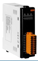
The USB-2045 is a full-speed USB device with 16 digital output channels module. The USB-2045 supports source type output and equips with short circuit protection. There are 16 LED indicators that can be used to monitor the status of the digital output channels. The 4 kV ESD protection, 0.5 kV EFT protection, 3 kV surge protection for power input and 3750 VDC Intra-module isolation are standard.
